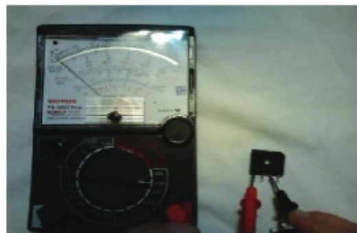
Step 4 Testing Bridge Rectifier IC
