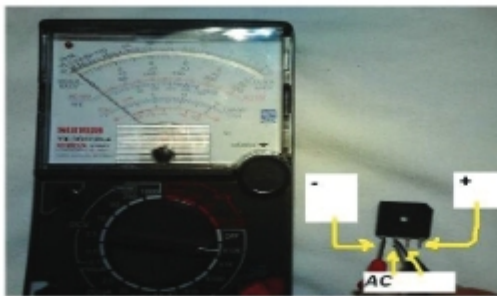
Step 1 Testing Bridge Rectifier IC
