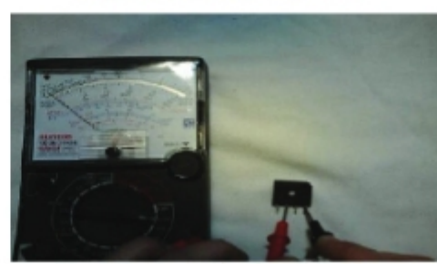
Step 8 Testing Bridge Rectifier IC
