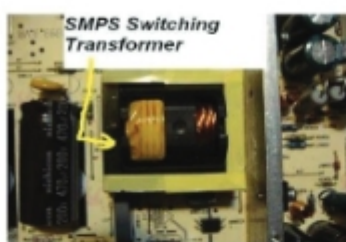
Switching Transformer In LCD TV PSU
