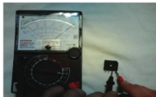
Step 6 Testing Bridge Rectifier IC
