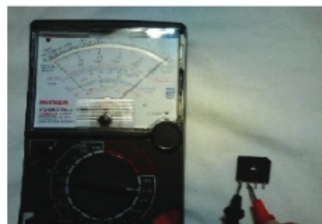
Step 2 Testing Bridge Rectifier IC
