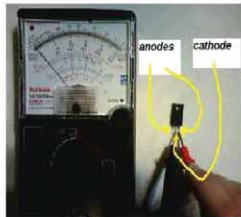
Step 4 Testing Schottky Diode In x1 ohm Setting
