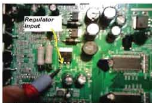
Checking Input Voltage to Regulator
