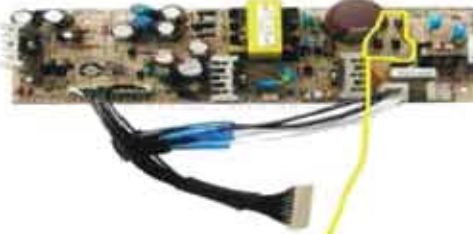
Four Diode Bridge In PSU
