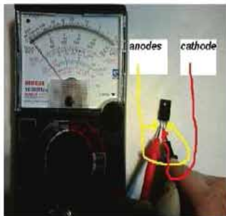
Step 3 Testing Schottky Diode In x1 ohm Setting
